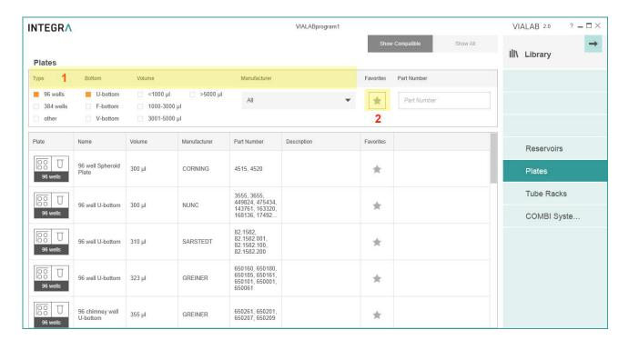
Select the desired properties or manufacturer (1) to quickly show reservoirs/plates/tube racks/COMBI Systems which are compatible with the selected pipette and deck position.
