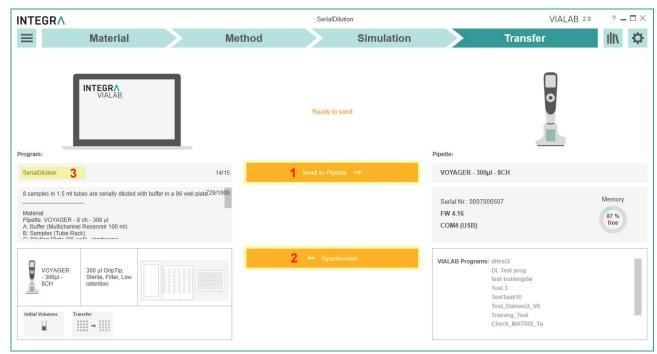
Send to Pipette (1) starts the transfer of the current program to the pipette. If certain parameters of the program are modified on the pipette (offsets, pipetting heights), synchronization of the program to VIALAB is possible (2).
