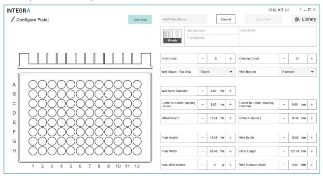
**Note:** For plates in adapters, e. g. in PCR 96 or 384 well cooling plates, define the dimensions of the inserted plate in combination with the adapter as one plate.
